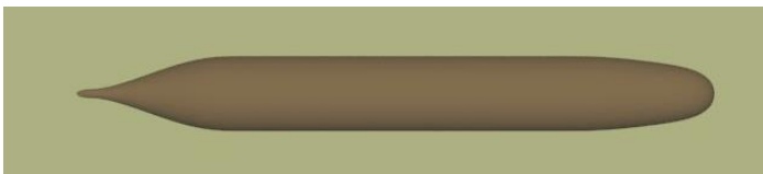
Figure 3. 3-D view of DARPA Suboff bare hull
