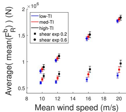
**FIGURE 6** Mean radial loading and standard deviations across each CPLS in DMB-1 model. Results are staggered about each wind-speed for clarity.
