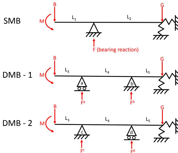
**FIGURE 3** Main-bearing models for each pair of in-plane force-moment pairs. Note that  $G$  is the gearbox weight in the vertical plane and zero in the horizontal plane.
