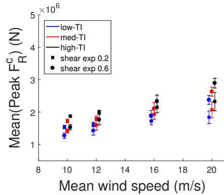
**FIGURE 11** Mean-peak radial loading and standard deviations across each CPLS in DMB-2 model. Results are staggered about each wind-speed for clarity.
