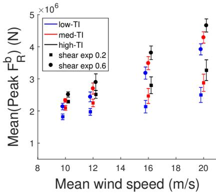
**FIGURE 10** Mean-peak radial loading and standard deviations across each CPLS in DMB-1 model. Results are staggered about each wind-speed for clarity.
