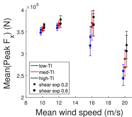
**FIGURE 8** Mean-peak axial loading and standard deviations across each CPL for all three models. Results are staggered about each mean wind-speed for clarity.
