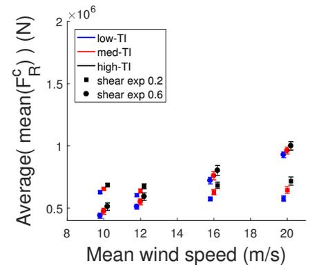
**FIGURE 7** Mean radial loading and standard deviations across each CPLS in DMB-2 model. Results are staggered about each wind-speed for clarity.
