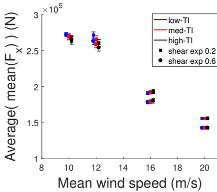
**FIGURE 4** Mean axial loading and standard deviations across each CPLS for the axial-reacting bearing in each of the three models. Results are staggered about each wind-speed for clarity.
