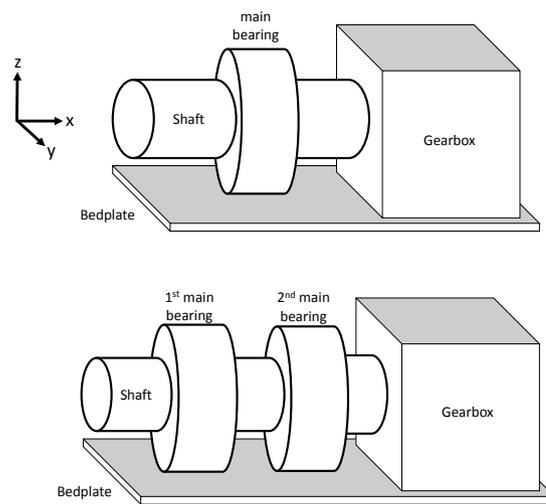
FIGURE 2 Main-bearing schematic for single and double bearing configurations. The reference frame is also given.
