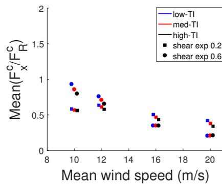
FIGURE 17 Mean load ratios across the spectrum of wind conditions for DMB-2 model. Results are staggered about each wind-speed for clarity.
