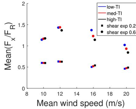
FIGURE 15 Mean load ratios across the spectrum of wind conditions for SMB model. Results are staggered about each wind-speed for clarity.
