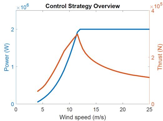
FIGURE 1 Turbine designed power and thrust curve against wind speed.
