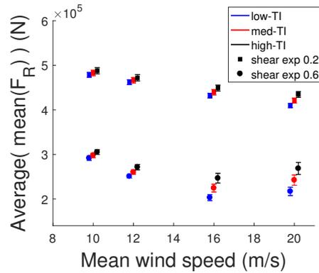
**FIGURE 5** Mean radial loading and standard deviations across each CPLS in SMB model. Results are staggered about each wind-speed for clarity.
