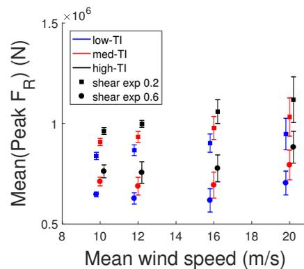
**FIGURE 9** Mean-peak radial loading and standard deviations across each CPL in SMB model. Results are staggered about each wind-speed for clarity.
