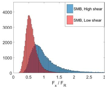
**FIGURE 12** Histograms of load ratios for SMB model in 10 m/s mean wind speed and medium TI.
