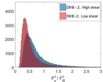
**FIGURE 14** Histograms of load ratios for DMB-2 model in 10 m/s mean wind speed and medium TI.
