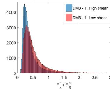
**FIGURE 13** Histograms of load ratios for DMB-1 model in 10 m/s mean wind speed and medium TI.
