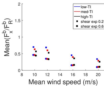
FIGURE 16 Mean load ratios across the spectrum of wind conditions for DMB-1 model. Results are staggered about each wind-speed for clarity.
