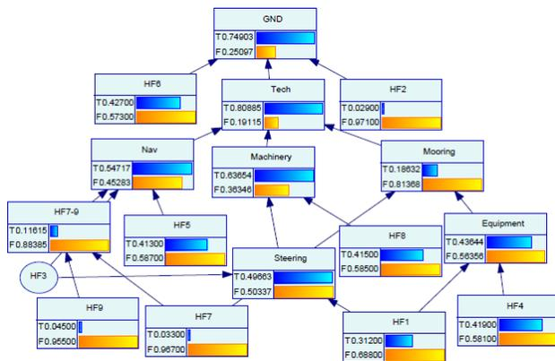
Figure 5. BN model for the wreckage/stranding accident.
