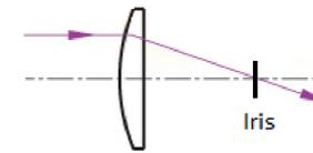
The convergence cannot be measured accurately using this method as the whole width of the beam does not pass through the same focal point.
