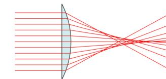
Bottom lens is a real lens showcasing spherical aberrations
