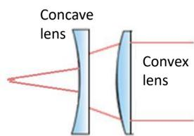
A laser beam can be expanded in size by using two lenses, a concave lens and then a convex. This lets you set the size and divergence of the beam.
