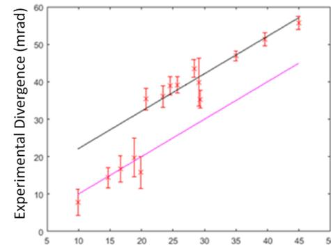
There is a 'jump' in the readings for the divergence. This is at the moment the beam goes from being clipped to unclipped.
