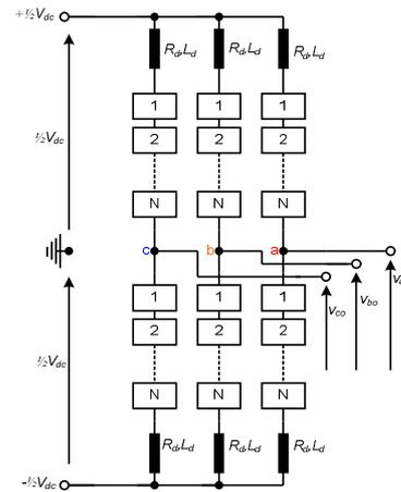
Fig. 1: Schematic diagrams of the generic MMC
