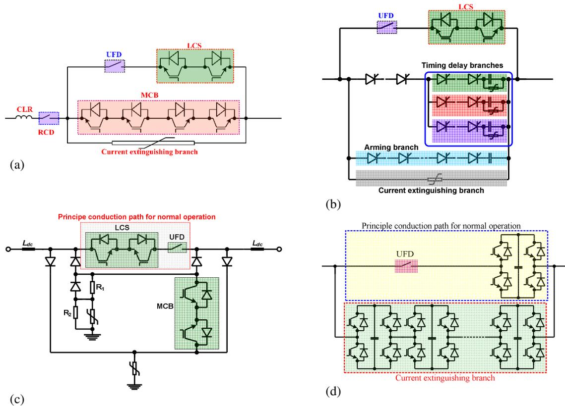
Fig. 6: Some hybrid dc circuit breakers being proposed for use for dc fault isolation in dc grids
