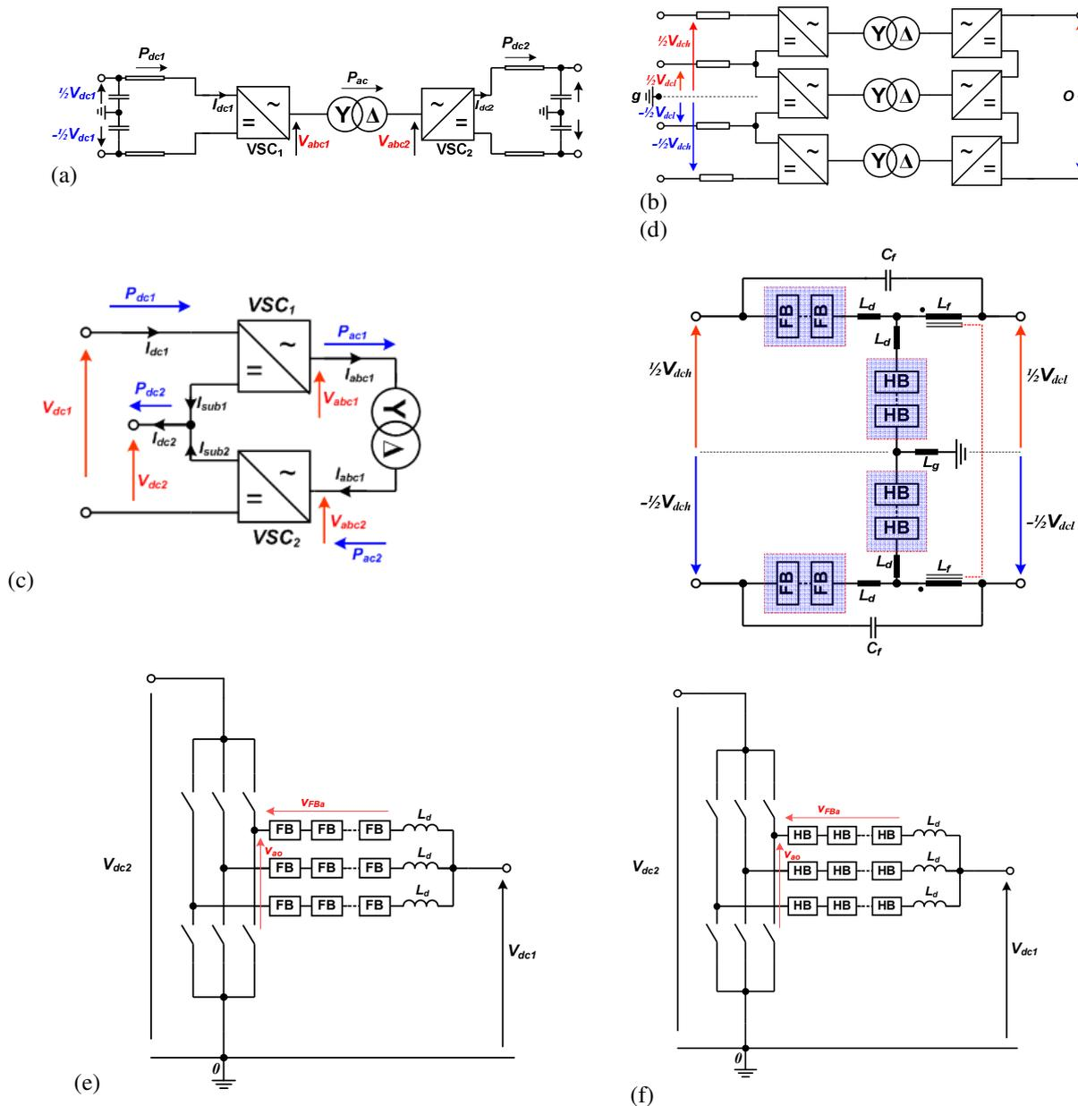
Fig. 4: Other examples of dc-dc converter topologies
