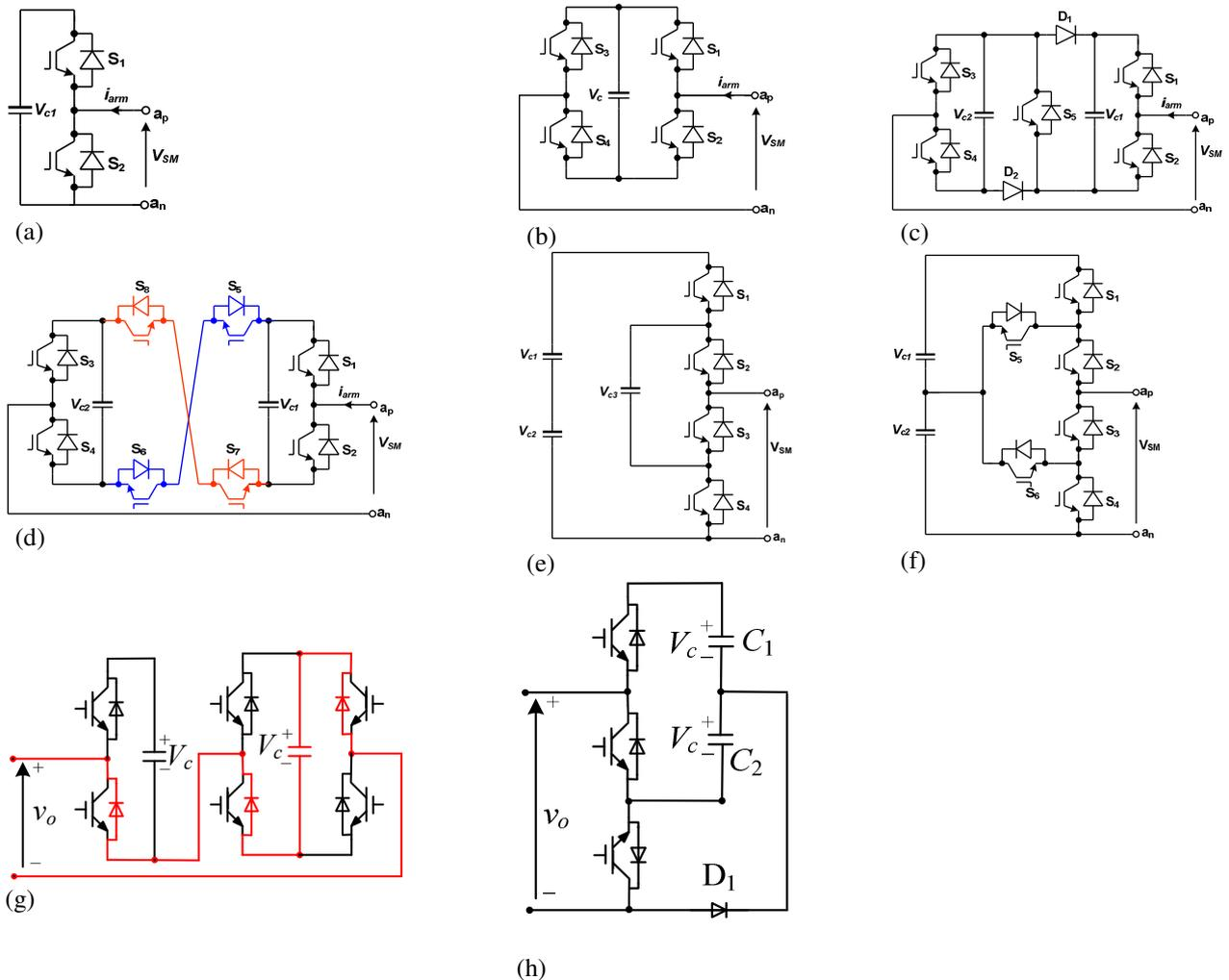
Fig. 2: Examples of MMC cells.
