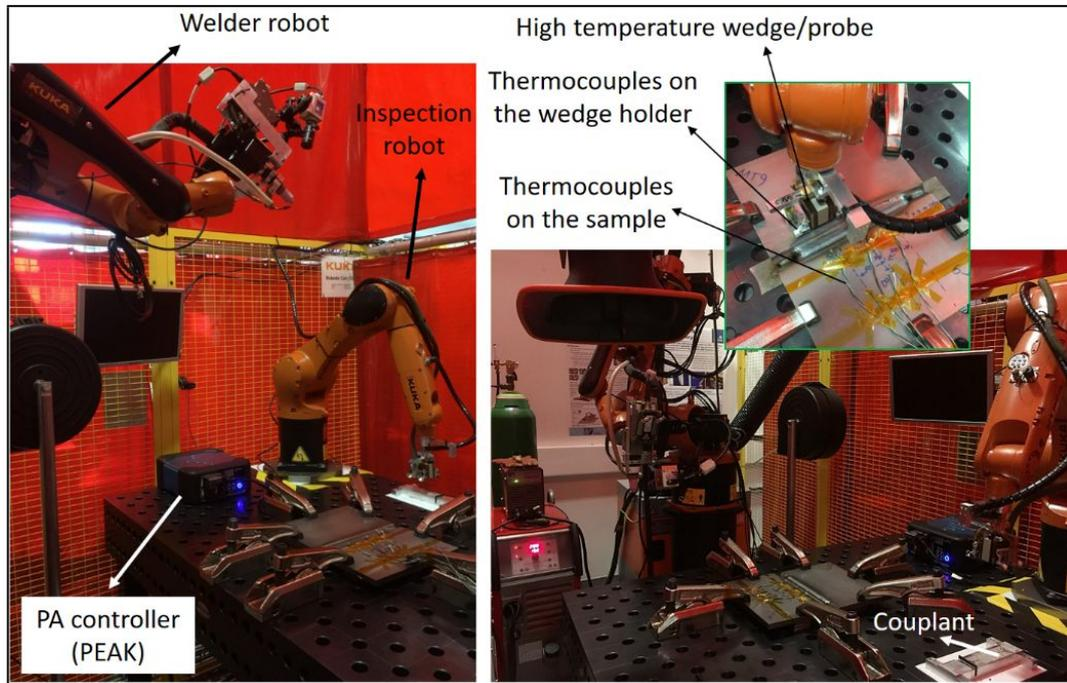
**Figure 1. In-process inspection of multi-pass robotic welding**
