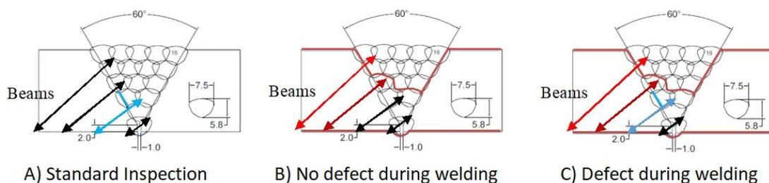
**Figure 6. Inspection configurations**
