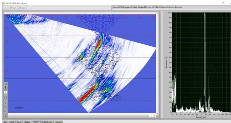
**Figure 5. Scan-converted image + overlay of pre-weld geometry and weld passes**
