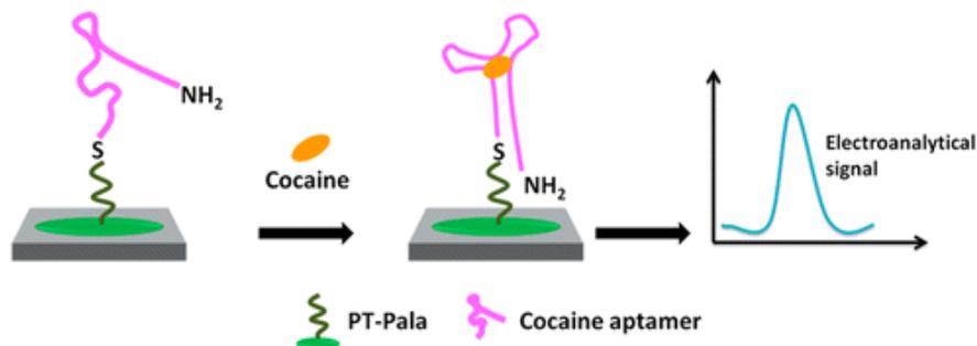
Figure 3: Schematic representing how a cocaine aptamer allows for cocaine detection. Reprinted with permission from Bozokalfa *et al.*<sup>47</sup> Copyright 2018 American Chemical Society.
