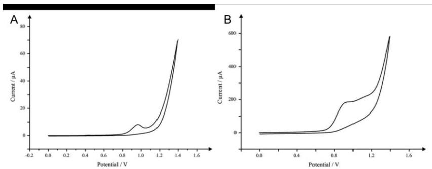
5 Figure 2: Typical cyclic voltammograms recorded at screen printed graphite electrochemical sensing platform vs SCE of (A) tonic water in the absence of atropine buffered to pH 10, scan rate  $50 \text{ mV s}^{-1}$  (B)  $1 \text{ mM}$  atropine in pH 10 buffer, scan rate  $100 \text{ mV s}^{-1}$ . (Reproduced from Ramdani et al.<sup>10</sup> with permission from The Royal Society of Chemistry)
