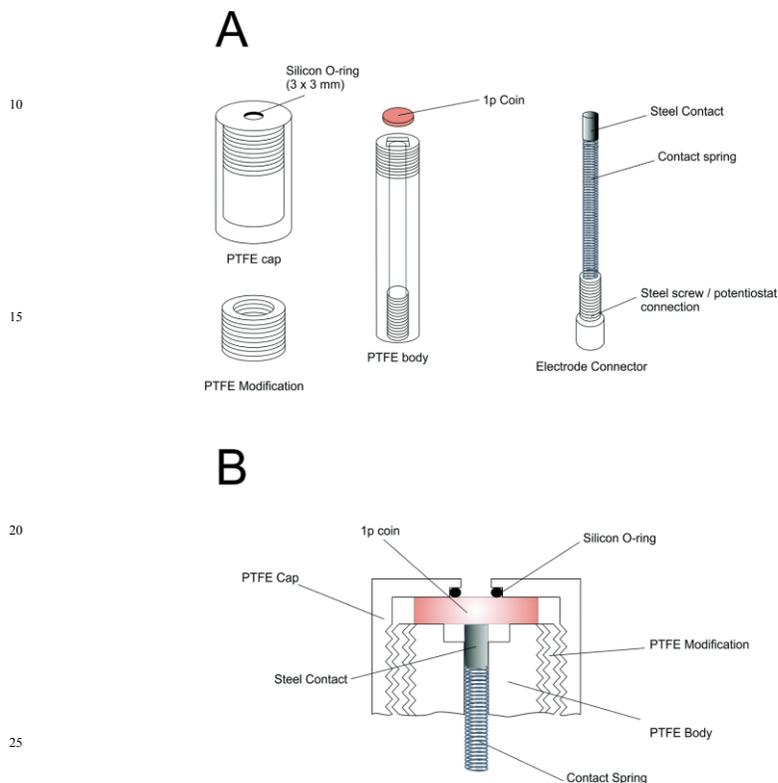
Figure 5: (A) Schematic diagram of the 1 pence coin working electrode construction, with the PTFE housing which holds the coin in place for analysis accurately defining the electrode area. (B) cross section of the assembled electrode which is then inserted into solution for analysis. Reproduced from Tan et al.<sup>53</sup> with permission from the Royal Society of Chemistry
