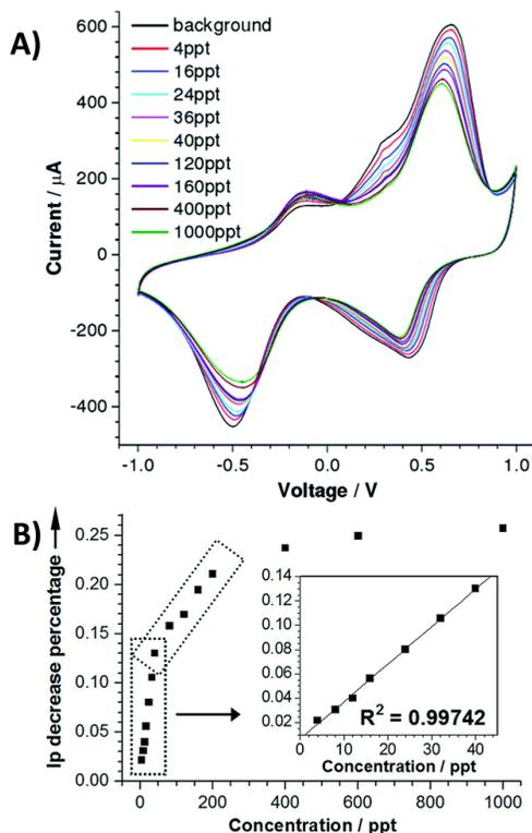
Figure 7: A) CVs obtained from the PANI/AuNPs/CNTs electrodes on addition of increasing concentrations of TNT, highlighting the decrease in anodic peak current at +0.65 V with a 0.5 M NaCl electrolyte and scan rate of 500  $\text{mV s}^{-1}$ . B) Calibration plot of anodic current percentage decrease against TNT concentration. Reproduced from Xi et al.<sup>63</sup> with permission from the Royal Society of Chemistry.
