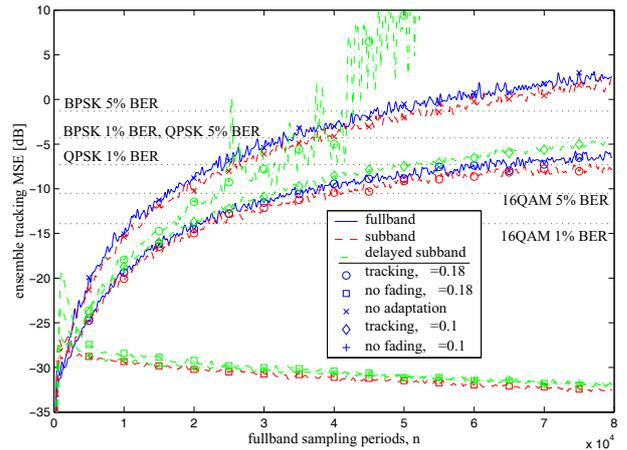
Figure 4: Channel-Equaliser Tracking MSE of a SS SV100M  $2 \times 2$  MIMO channel.
