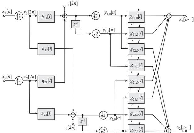
Figure 1: A polyphase representation of a  $2 \times 2$  MIMO  $T/2$  fractionally-spaced channel-equaliser system.
