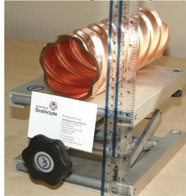
**Figure 6.** A section (6-periods) of 5-fold waveguide.
