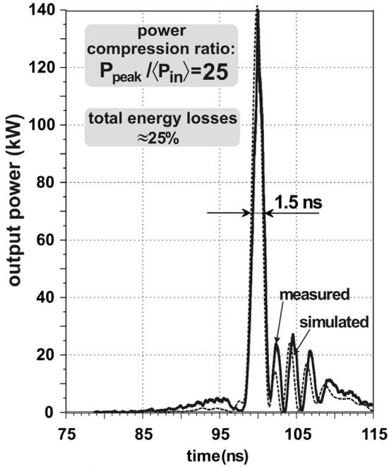
**Figure 3.** Measured (solid line) and simulated (dashed line) compressed pulse.
