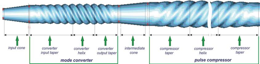
**Figure 4.** 5-fold microwave compressor set-up
