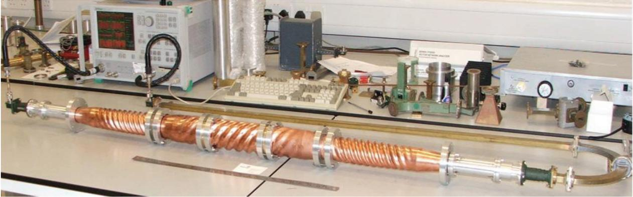
**Figure 7.** Photograph of the 5-fold compressor and VNA measurement system
