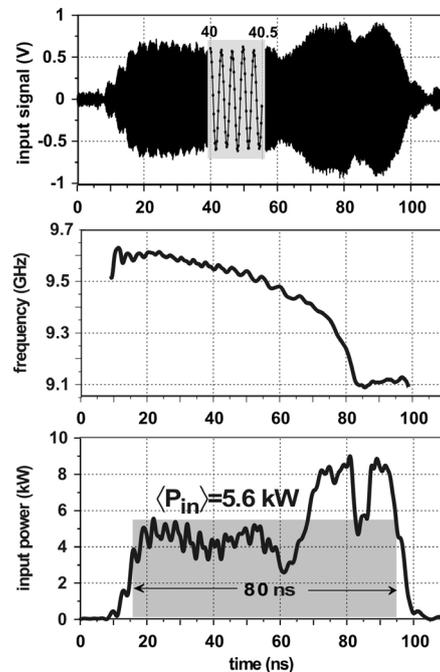
Figure 2. Input pulse details for pulse compression experiment.
