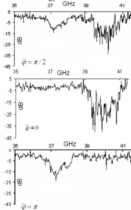
Figure 8: effect of changing the phase between 1D Bragg mirrors on the transmission profile.
