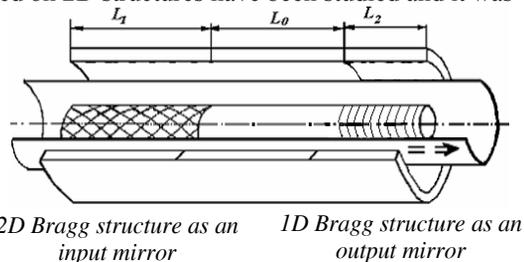
Figure 1: The schematic diagram of the FEM based on a combined two-mirror cavity.
