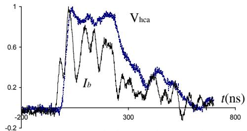
Figure 2: The measured electron beam voltage  $V_{hca}$  and current  $I_b$  plotted in normalised units
