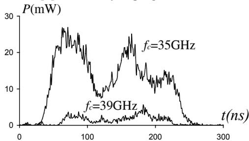
Figure 5: The RF pulse traces when the cut off filters are used
