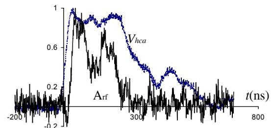
Figure 3: The measured electron beam voltage  $V_{hca}$  and microwave signal  $A_{rf}$  plotted in normalised units
