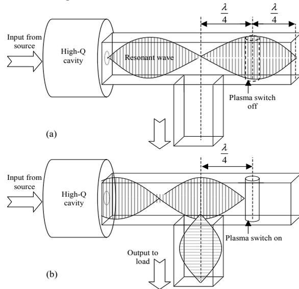
Figure 6: (a) resonant wave condition when the plasma switch is inactive (b) same arrangement with the plasma switch activated.
