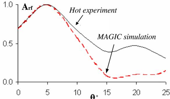
Figure 4: Mode pattern from the output horn measured in experiments (solid line) and simulations (dashed line).
