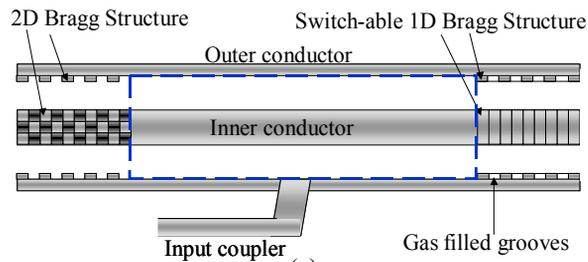
Figure 7: Schematic of the proposed SPBG pulse compressor cavity
