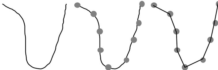
**Figure 3 Approximation of a curve by 8-element polyline.**
